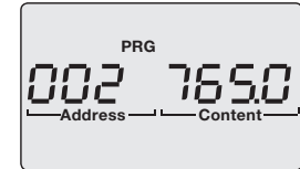
Display example 1: The primary voltage of each voltage transformer on the 4 voltage measurement inputs is 765 V.
